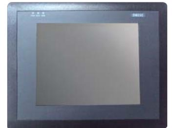
The microprocessor touch screen control can be programmed to display in four languages.
