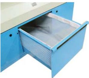
Large self-cleaning lint screens make maintenance easy. The screens are accessible from the front and located close to the exhaust fan, preventing fan clog up and eliminating fan vibrations. The lint filter is efficient and provides a good airflow that reduces the energy consumption. The microprocessor monitors the lint filter and stops the machine, should the lint screen become blocked.
