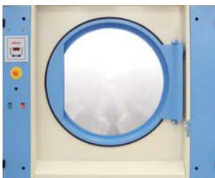
The large door opens 180 degrees making loading and unloading easy. The door glass is attached to the door without any gasket providing a long lasting door that offers security and low maintenance over the life of the machine. The door is provided with a safety switch that stops the machine when the door is open. A magnetic latch holds the door closed during operation. The door can be opened any time during operation for safety.
