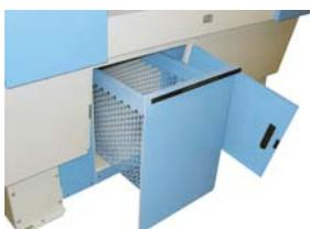
A large dual lint compartment makes maintenance easy. It is accessible from the front and located close to the exhaust fan, preventing fan clog up and eliminating fan vibrations. The lint filter is efficient and provides a good airflow that reduces energy consumption. The microprocessor monitors the lint filter and stops the machine, should the lint screen become blocked.
